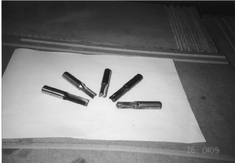
Fig. 9. TCT panel cutters with different tool wear states.
